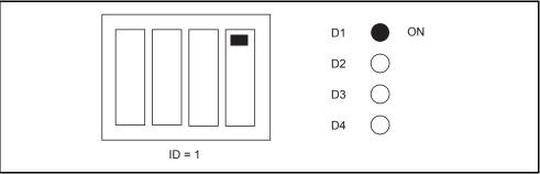
After 10 seconds, the address of the TankGate will be set to the ID DIP Switch setting. The LEDS will flash for 5 seconds to indicate that the address is about to be set.
